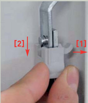
Release the 2 linking rings from the connecting rods and the mechanism
