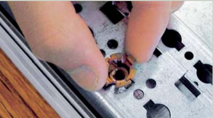
Two clip-nuts (provided) are sufficient to hold all versions of plates
