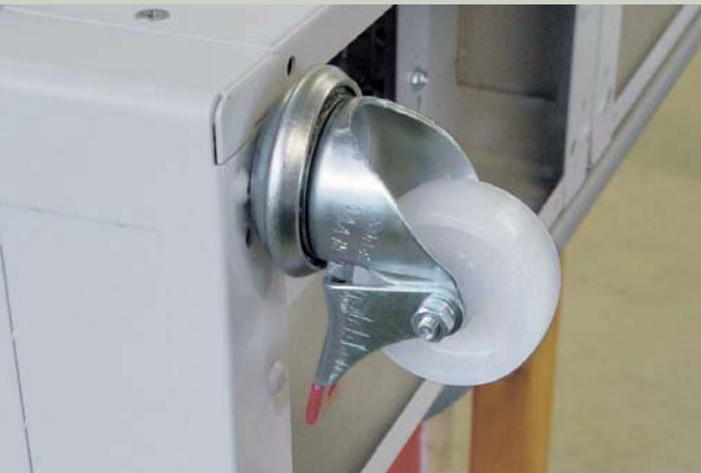
Castors Cat. No. 347 93 are fixed directly on the plinths of the enclosures boring 12 mm holes
