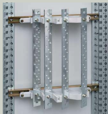
Fix the distribution block on the rails using hammer head bolts Cat. No. 367 60.
