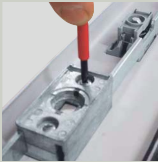
Unscrew the 2 screws fixing the handle and the mechanism
