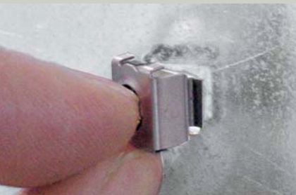
Fitting the cage nuts, via the rear of the metal plate
