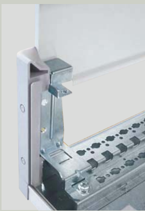
Slide the side panels steadily in the corner runners until they are inserted in the back
