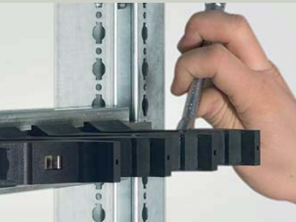
Fix the support using M6 screws (tightening torque 10 Nm)
