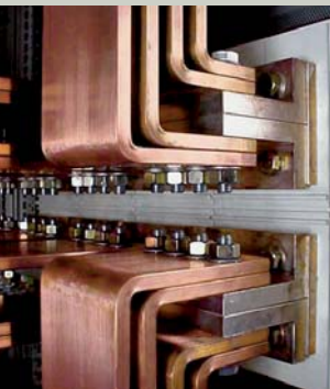
Connection of four 100 x 10 bars on each rear terminal of a draw-out DMX 4000
