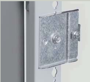
Fix the 4 "lug + hinge" assemblies on the back of the structural upright using clip-nuts and M6 screws
