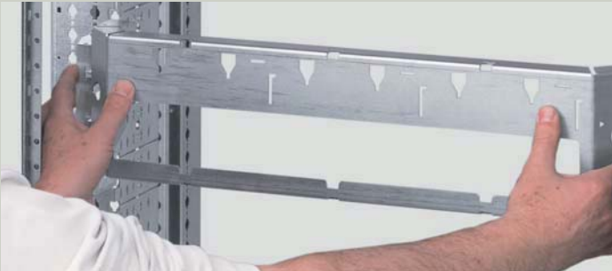
Slide the plate to the required position
