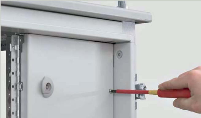
Fix the front cover on the hinges using the countersunk head screws provided, then insert the plastic covers in the screw heads to improve the finish
