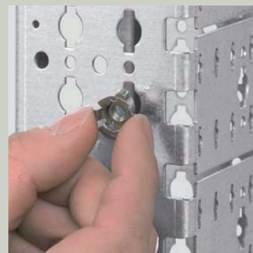
Fitting the clip-nuts
