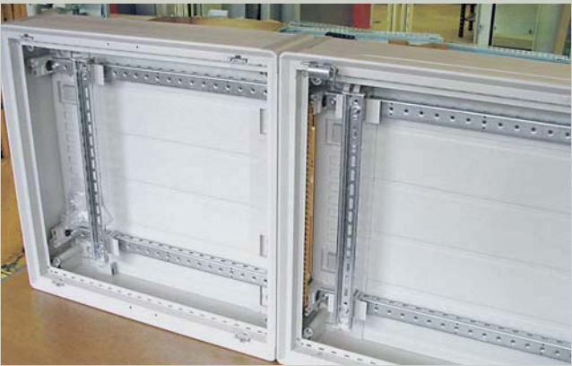
Position the enclosures on their sides to align them perfectly, then carry out the final tightening
