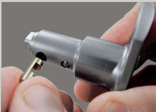
Insert the pin in the notch towards the front
