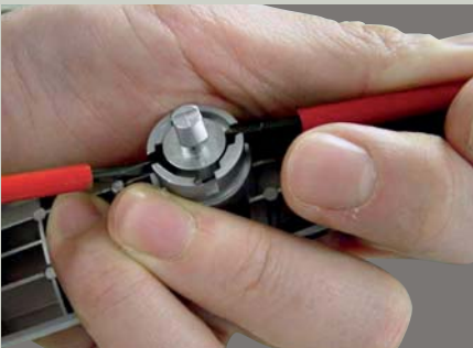
Push in the 2 black clips to remove the blanking plate
