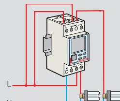
Output closing and breaking times are calculated based on the date, the actual time when the device was switched and on geographical coordinates of the actual location
