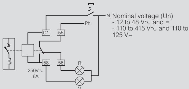
Equipped with a signalling contact which indicates tripping of the shunt trip and automatically breaks the coil.
