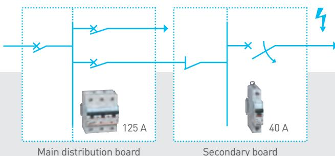
The tripping characteristics are calculated and adjusted to ensure correct discrimination between the different protection levels in order to improve ease of use.
