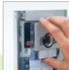
3 Loosen the clips and slip off the front plate
